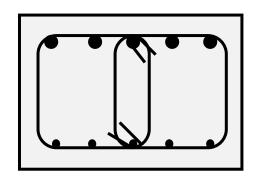
Top reinforcement is lap-spliced at midspan, bottom reinforcement is lap-spliced over supports
